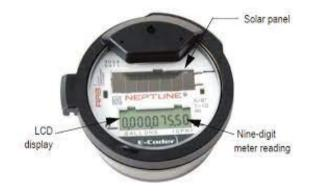
When the LCD displays the reading it will have seven numbers before the decimal point and two after. The numbers before the decimal point are whole numbers and after the decimal point are the fractions of a gallon. For example the reading below is Thirty-three thousand, Eighty -nine and a quarter of a gallon. We only read a thousand and above, so the reading would be 33.
